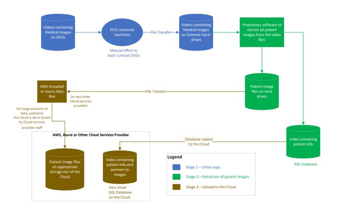
As shown in the above diagram, the images are extracted from the CDs / DVDs and uploaded to the Cloud (or a network drive in your datacenter) in three stages.
